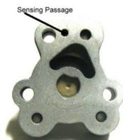
Before the final assembly of the adjustable bypass valve, the adjustment screw, spring washer and adjustment nut are assembled into the larger casting. The initial adjustment should position the nut about one screw turn after it enters the hex section of the casting. This is the minimum sensitivity position and keep should keep the valve firmly closed during initial carb tuning.
