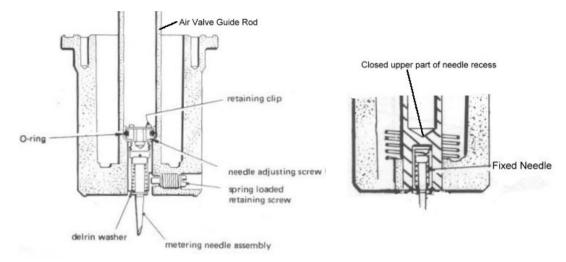
The sketches above show the air valve with adjustable needle on the left and fixed needle on the right. The needle recess for the fixed needle is smaller than for the fixed needle and sealed at the top.
