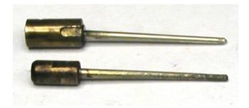
**Needle Recess:** Careful inspection of the fixed needle air valve revealed that if the needle recess were enlarged and the closed upper portion drilled out, this area of the two valves would be identical. Of special importance was that the position of the shoulder where the lower side of the lip on the adjustment screw rests is the same in both the adjustable needle air valve and the fixed needle valve.
