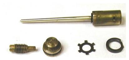
The photo above shows the adjustable needle with needle retaining screw, adjustment screw, adjustment screw retaining clip and an old damage O rig that fits in the slot on the adjustment screw. The photo below shows a comparison of the adjustable needle with the larger carrier and the fixed needle with the smaller carrier. The actual needles are essentially identical.
