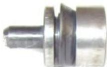
The first step in the rebuild is to put the new rubber seal on the new piston. Before doing this, apply a little rubber grease to the back of the piston to allow the seal to be slid on without damage. The largest part of the seal should be towards the closed end of the cylinder (front of the car) as shown in photo.
