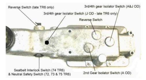
**Reverse Switch:** The reverse switch is linked to the left most selector shaft that controls the reverse gear. The reverse switch operates when the gearbox is shifted into reverse to turn on the backup lamps. The switch is located on the top left side near the front of the cover in pre '74 gearboxes. The switch is on the left side near the rear on the '74 and later gearboxes.
