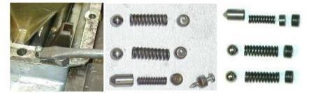
I was unable to get replacement pressed- in plugs for the '76 but was able to get the older threaded style from TRF, which were used. After the selectors were removed, the three holes were tapped 7/16-20. The existing holes were the correct size so all I had to do was find the tap and use it. The photo below shows a hole being tapped. This occurred much later in the process but I thought it better to show here to wrap up this subject.
