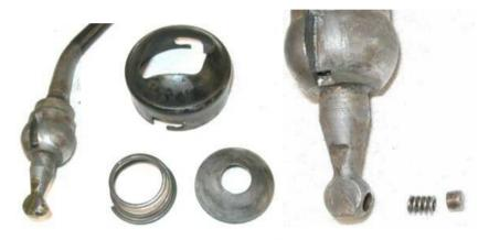
The TR3 & TR4 gearboxes used a different cap then the later gearboxes. The photo below is of parts from a TR4 gearbox and is similar to that on that for the TR3 except that the TR3 shifter is straight. Note the bolt that goes though a hole in the bottom of the shift lever and both side holes in the cap.
