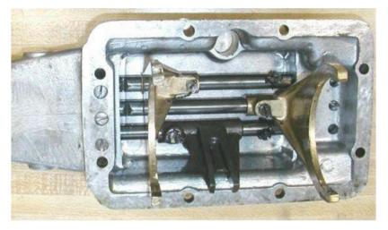
**Removing the selectors:** The square headed tapered screws securing the forks to the selector shafts were difficult to remove. A good quality 12 point 3/8 socket as shown in an earlier photo was used. That worked for five of the screws. One of the heads had the corners rounded a little and the socket slipped so I had to resort to a 5/16 open-end wrench for that one.
