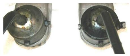
The procedure to install the cap with the shifters that use the long retaining bolt is similar to above, except that that long bolt that goes thorough the hole in the shifter rather than the small bolt at the rear secures the cap. No adjustment is required in this case.
