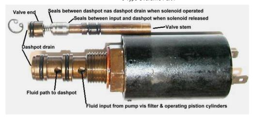
Relief Valve & Dashpot: The photo at right shows the dashpot and part of the relief valve being removed from the main casting. The plug was removed first and laid face up on the casting.
