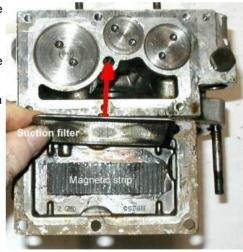
**The Pump:** The photo on the right shows the front of the main casting. The pump is in the lower part. The pump piston is pulled up and pushed down by the cam follower as the mainshaft and attached cam rotate. The pump piston, pin, cam and cylinder are steel. The Cam follower and the main casting are aluminum.
