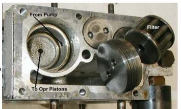
**Operating Pistons:** The operating pistons are located in the main casting as shown in the photo on right. The left piston has been removed. Note the rubber O-Rring used to seal the piston. The fluid entry and exit holes for the left cylinder are indicated on the photo.
