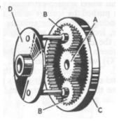
The operation of these gears is not obvious (at least to me) at first glance. The four things to remember when trying to understand the epicyclic gear are:
