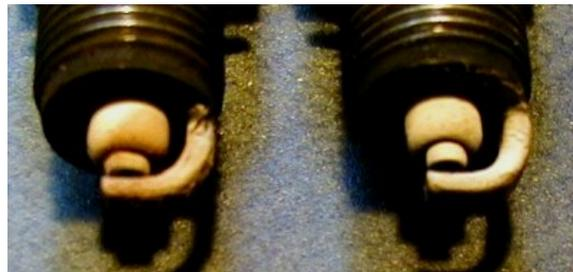
Two plugs with the brownish color indicating carbs with a properly adjusted mixture. All the plugs shown are Champion N12Cs.
