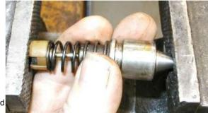
After the secondary piston was back together I slid the new seal onto the piston as shown on the right. This one was much easier to install than the one on the primary piston.
