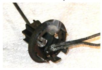
Once the joint is hot, the solder is touched to the joint and held till a small amount flows into the crack between the two metals, see next photo.
