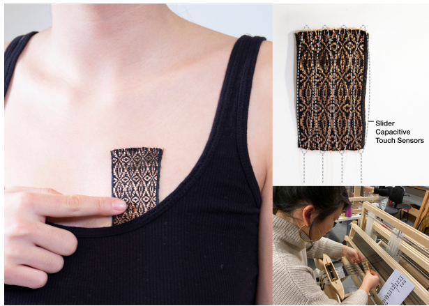
Figure 8. Skylar's WovenSkin device: A capacitive touch slider for "touching one's own heart" woven with overshot patterns.
