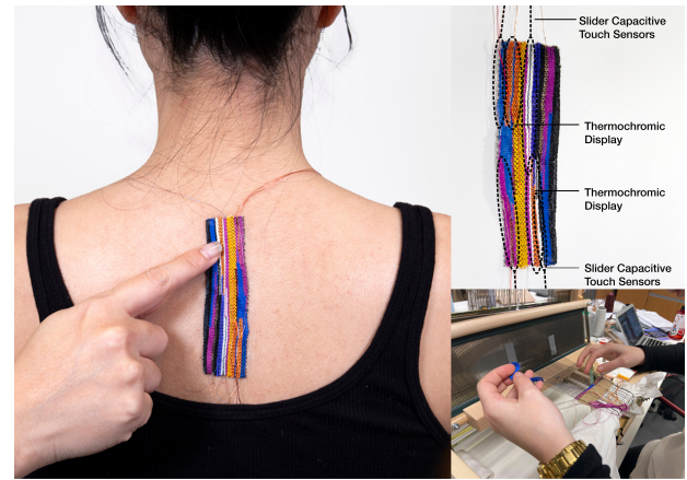
Figure 9. Quinn's WovenSkin device: A drawing interface for social interaction. When someone touches the interface, it changes color while projecting the touch input on a phone or laptop screen so the wearer could see it.
