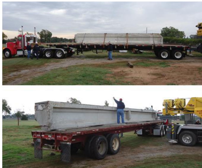
Figure 1: Two full-scale girders being delivered for testing, Girder A (top) and Girder C (bottom)
