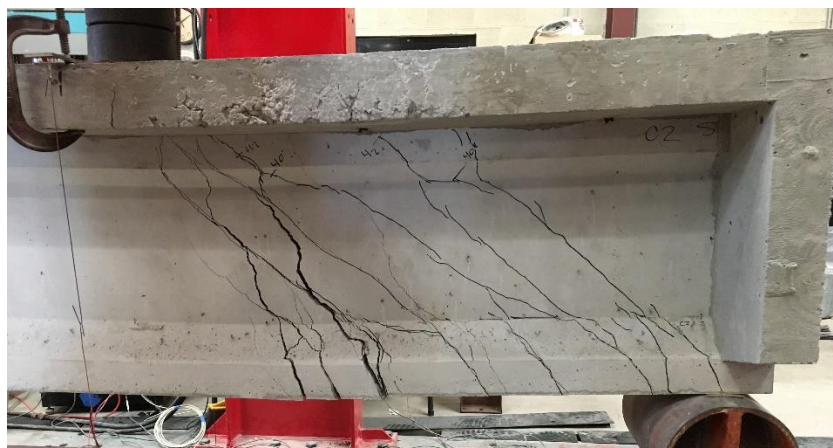
Figure 10: Girder C2s failure
