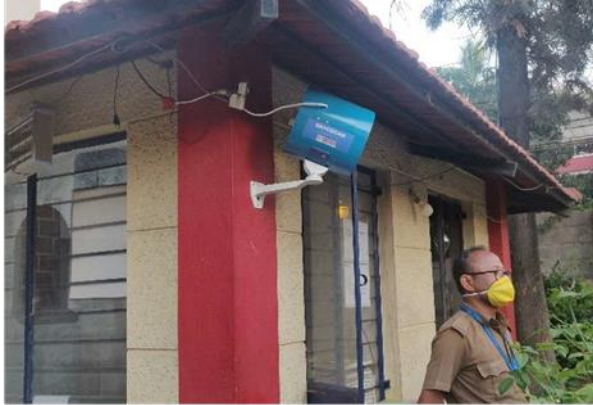
Fig. 2 Prototype of the device Scalene Hypercharge Corona Canon (SHYCOCAN) for reduction of Infectivity and prevention of air and surface borne transmission of COVID-19 – Installed at our Campus Security department.
