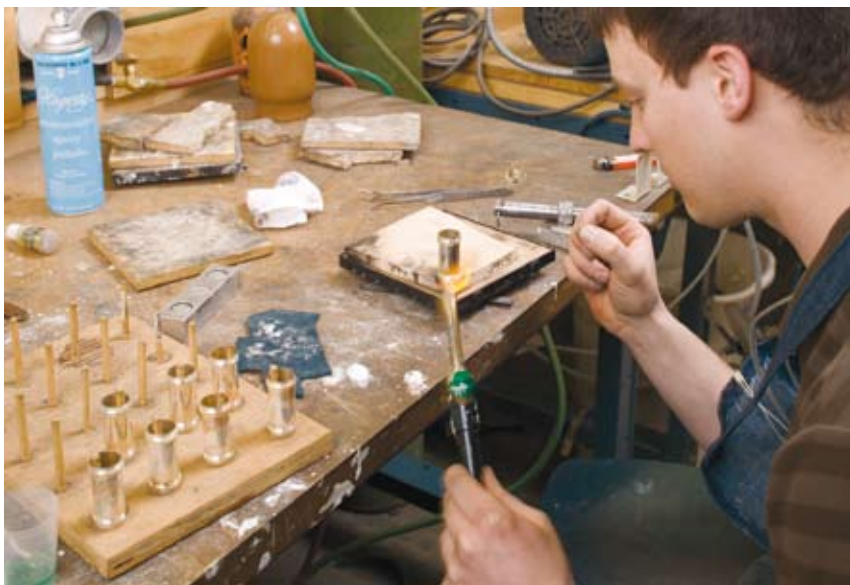
Soldering ferrules to a socket before soldering the socket to the flute body.
