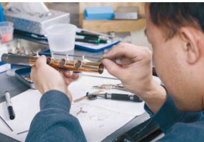
Checking the alignment of the pillars.
