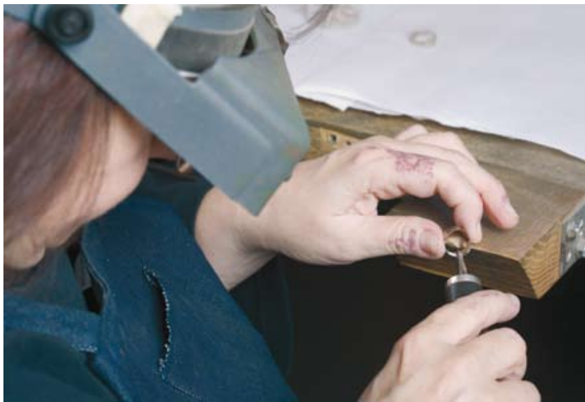
Preparing a tonehole for soldering onto a flute body.
