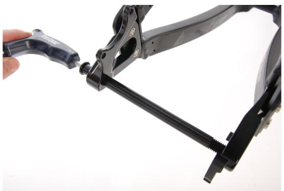
3: Apply grease to the rear axle and threads. Once wheel is installed, torque axle to 8Nm.
