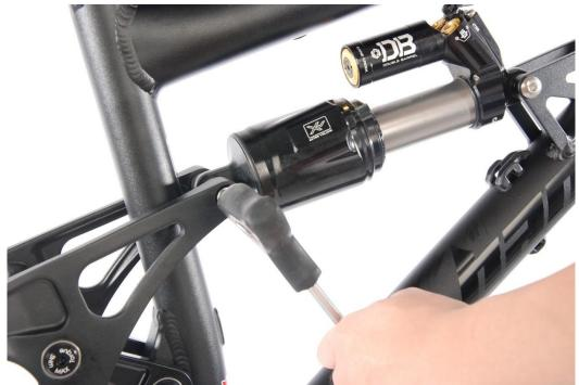
10: Apply blue Loctite to shock bolts and reinsert the rear shock.
