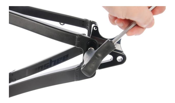
2: Install the flip chips and the dropout bolts onto the rear triangle with the rear axle loosely in place to ensure good alignment initially. Torque to 12Nm.
