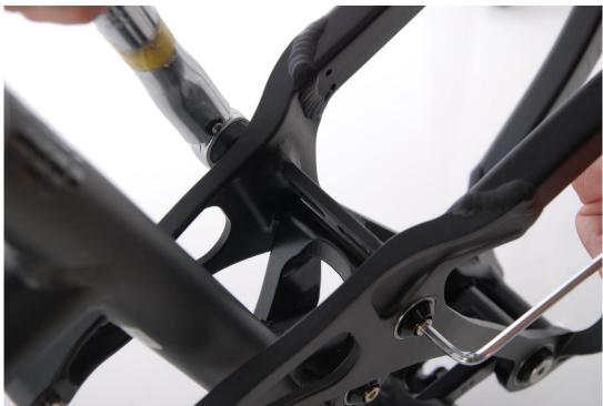
9: Lightly grease the pivot axles and reinsert them into the frame. Prepare the threads of all axle bolts with blue Loctite. Using two allen keys, tighten the pivot axle bolts. Use a torque wrench and confirm that it is torqued to no greater than marked on the pivot axle or bolt being tightened.
