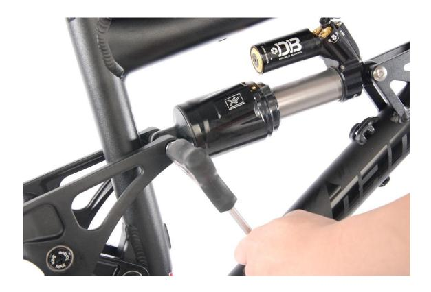
1: Remove the shock from the frame using a single 6mm allen key at the rear and two 5mm allen keys at the front.
