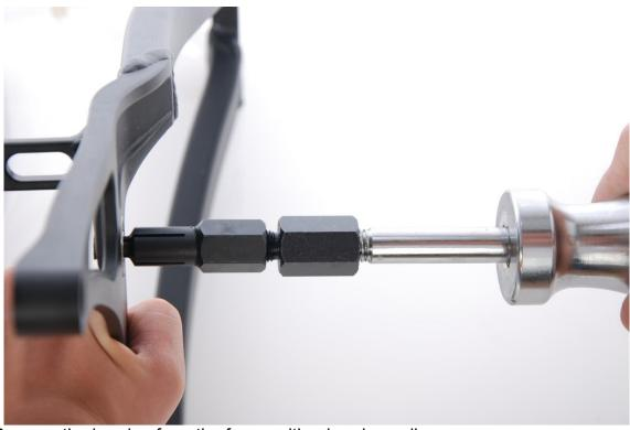
6: Remove the bearing from the frame with a bearing puller.
