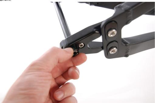
4: Apply a dab of blue loctite to axle lock bolt. Install the rear axle bolt, torque to a maximum of 3Nm. (this bolt is not structural, it is purely to prevent the axle from working loose) Be careful not to over-tighten this bolt otherwise it may be damaged.
