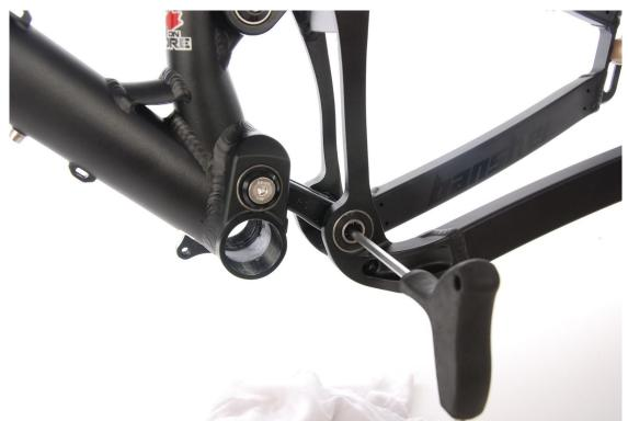
5: Remove the pivot axles by sliding them out of the frame. If an axle is difficult to remove, use a punch or allen key that fits inside the hollow axle, and tap it out being careful not to damage axle threads.
