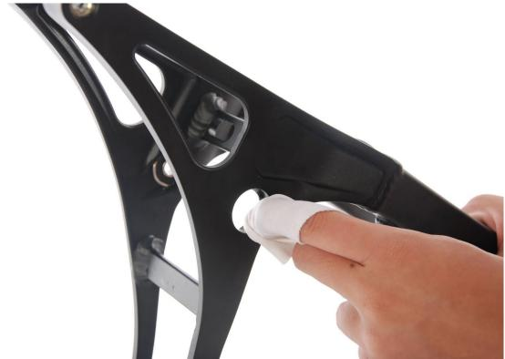
7: Clean and inspect the frame once the bearings are removed.
