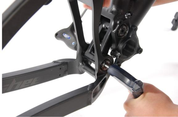
3: Remove the pivot bolt hardware from the frame using appropriate allen keys.
