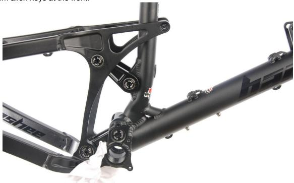
2: Stuff a rag under the bottom link to prevent damages to the frame.
