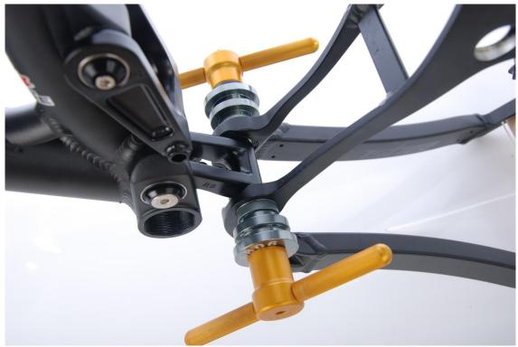
8: Press the bearings into the frame using a bearing press.
