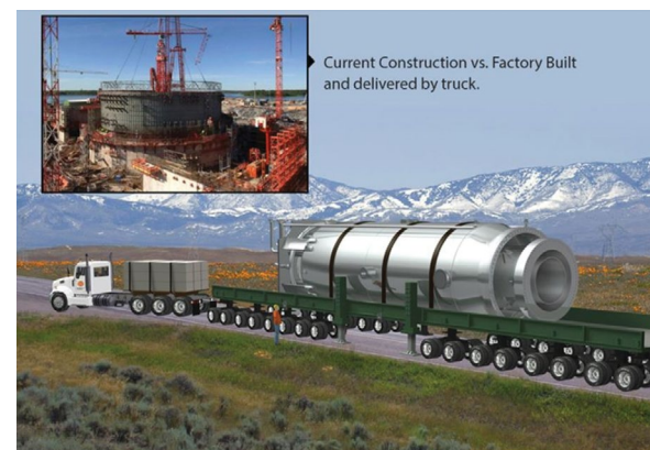
Figure 48. An illustration highlighting the differences between the physical size and construction of a traditional nuclear power plant and a small modular reactor (Source: Power Technology )
