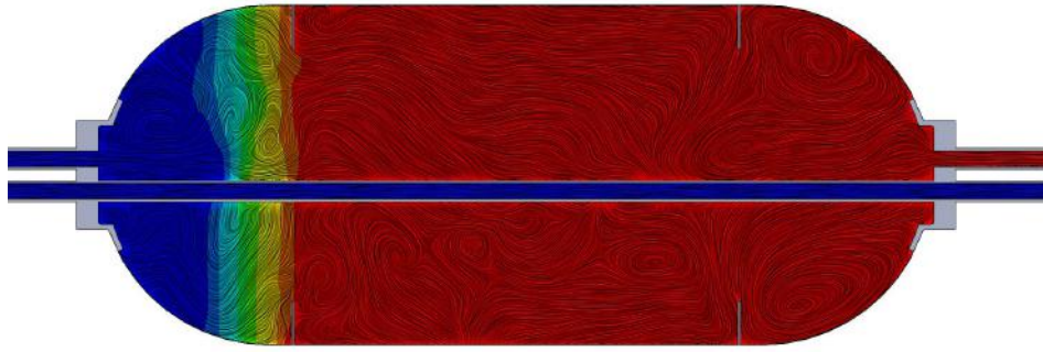
Figure 4.16: Fluid velocity within the RP1 tank with fluid level near top baffle
