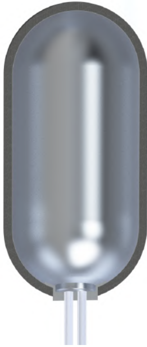
Figure 4.19: Final RP1 tank design
