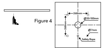
**3.** Fix another side of safety rope on the ceiling, then connect the wire of fixture to main supply according to local electrical connection mode, make sure good protection on the wire joint, after that, fix the fixture on the ceiling with accessory screws (Figfure 5).
