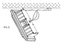
4. Buckle the fixture completely on the mounting bracket; Fix side screws of bracket on the fixture. See picture 4.
