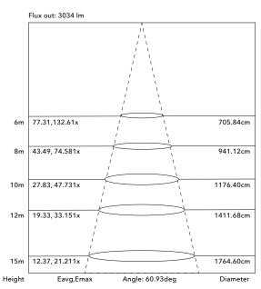
Note: The Curves indicate the illuminated area and the average ilumination when the luminaire is at different distance.
