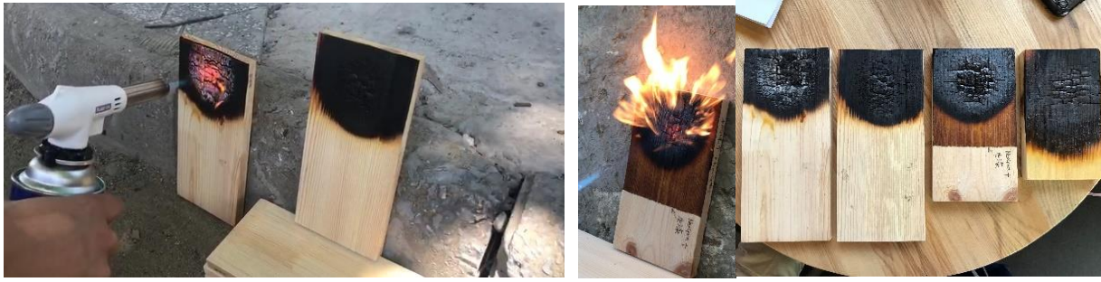
Fig. 9. Fireproof Paint Test (self-photography)
