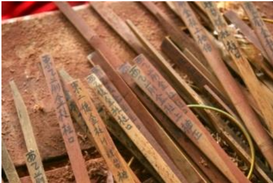
Fig. 32. Tool of Zhaomian for the spiral zaojing in Ninghai © Yaping Zhang
