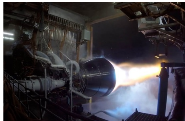
The hot fire test of Blue Origin's BE-4 engine.
