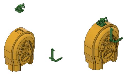
Regulator fits into the firebox backhead and steam manifold goes on top.
