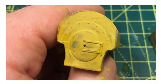
The front of the saddle tank section of an Avonside B4 kit after a coat of filler primer and some fine wet and dry sandpaper (used wet) - note that the primer has filled in the gaps in the layers
