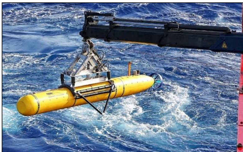
Artemis - A 5,000 Meter rated autonomous underwater vehicle
