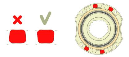
Close OCHAIN referring to lasered alignment marks "♣"
