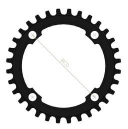
\*\*Bolt Circle Diameter or BCD is the imaginary circle that passes through the center of all the chainring mounting holes.
