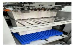
The pallets can be used throughout the production process. Printing and die cutting can benefit from "none stop" feeding of board/paper/ corrugated using swords on the feeder.
