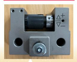
Optimising your die cutter performance is essential. Being able to maximise your up time by adjusting the thin plate for the exact fit in relation to the cutting die for perfect creasing and embossing on repeat orders, is a key component of make ready speed. C&T are pleased to announce the addition of micro metric blocks for thin plate systems. We offer both operator and drive side, that fit all die cutting formats
