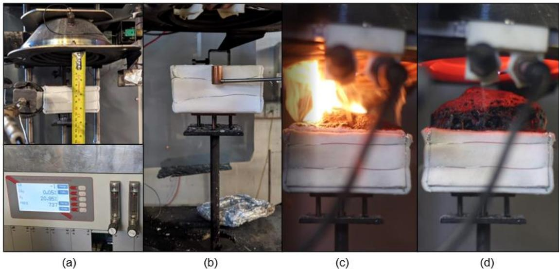
**Figure 4-3** Cone calorimeter test steps
