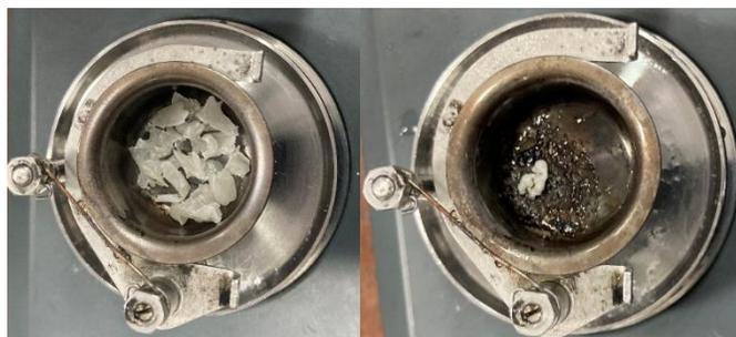
**Figure 5-25** Bomb calorimeter sample pictures before and after the experiment.
