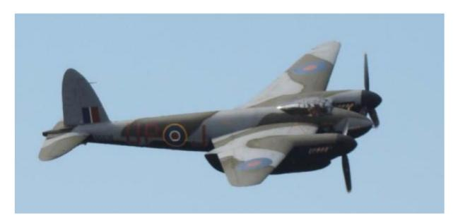
De Havilland Mosquito, also known as the 'Wooden Wonder' designed to be constructed from widely available plywood rather than aluminium, which was in short supply. Equipped with two Merlin engines this aircraft one of the fastest and most effective fighter-bombers of WW2
