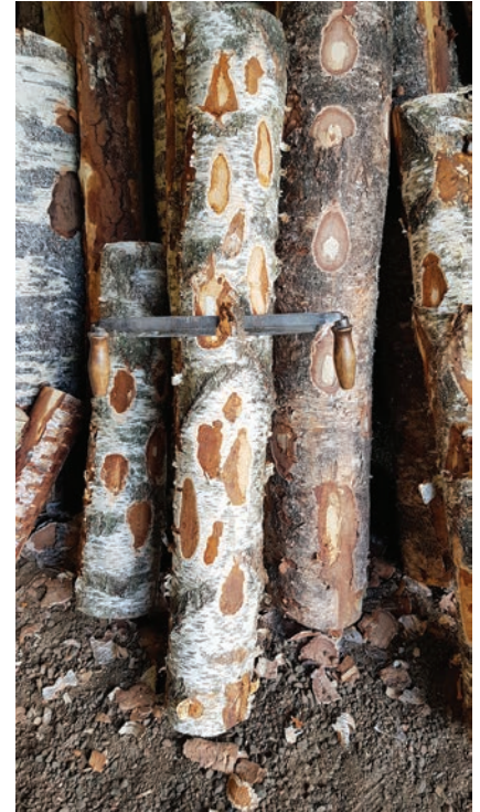
Fig. 1 After drying the complete tree for some months the trunk is cut into 2 m pieces and moved inside a barn. Pieces of the bark are removed around the trunk, using a draw knife. The subsequent drying will be slow with the trunks standing.
