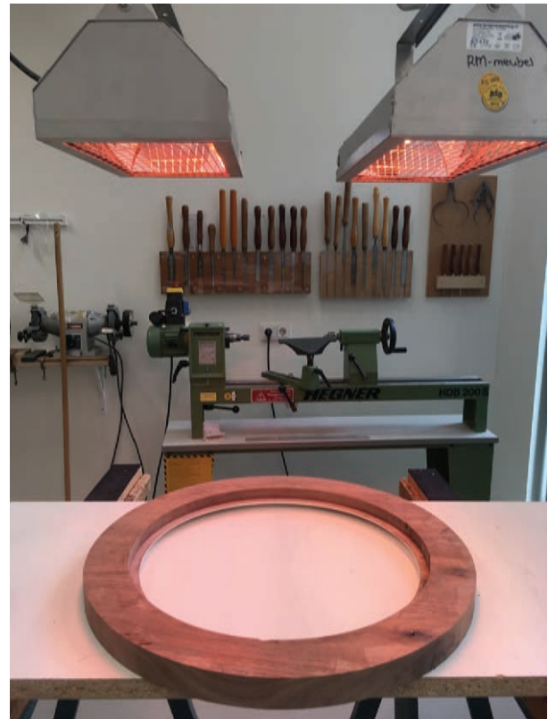
Fig. 16 Two infrared lamps used to heat the backside of the frame. © The author.
