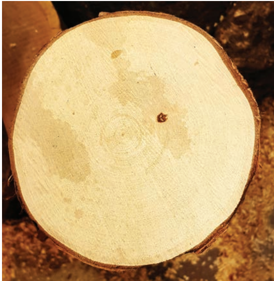
Fig. 2 The result from the summer-felling of a birch is a tough material, excellent for turning.
