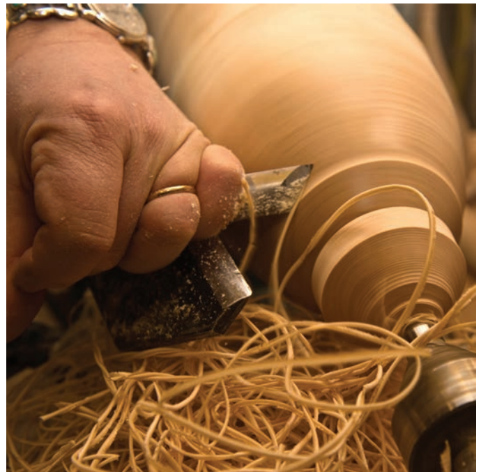
Fig. 5 The skew is cutting a beautiful shaving and producing a surface that made both the woodturner and customer happy. The low turning speed assures safe turning as only a low force is needed – provided that the tool is sharpened in a correct way.
