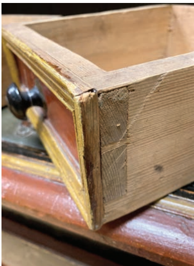
Fig. 7 The pins of a dovetail joint are normally put at right angles to the pushing and pulling direction of a drawer. This might however not always be the case as in the construction of a drawer in this vernacular cupboard from the early 19th century. Nordiska museet. Photo Johan Knutsson.
