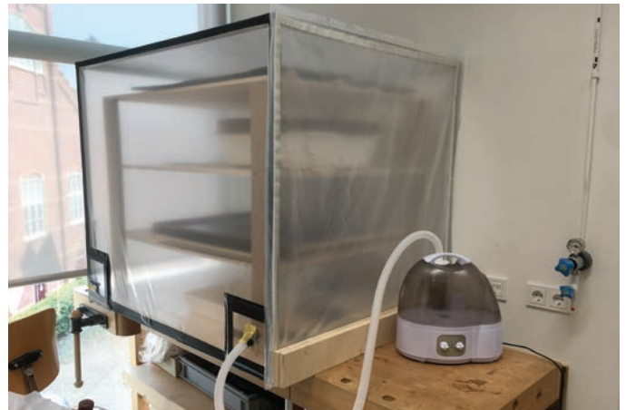
Fig. 15 Sealed climate chamber with thermostatic humidifier. © The author.
