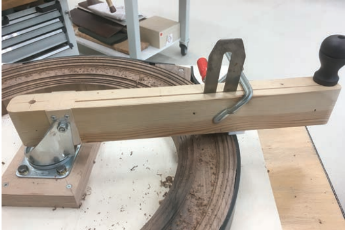
Fig. 10 The rotating pivoting system with scraping blade fixed to the lever. © The author.
