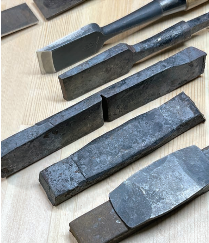
Fig. 2 A processing sample where steel is forged to the base metal. Image by Kenji Komatsu.
