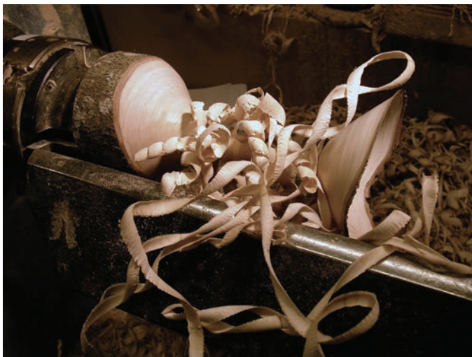
Fig. 4 The shaving “dancing” away from a wide, sharp, chisel resting on a slowly rotating chunk of wood produces a high-quality surface. This is one of 38 unique pieces being turned to show the soul of different trees. No sanding was done as that would have torn the soul!
