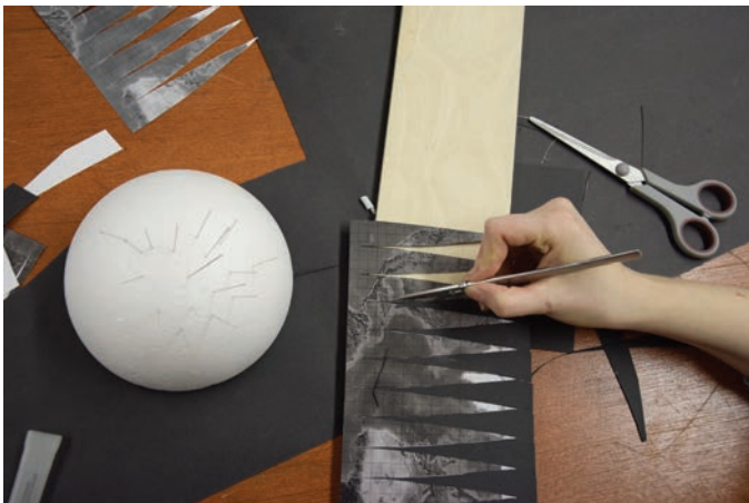
Fig. 8 Preparing the veneer for the spherical upper part of the conch. Image by L. Lessinger.
