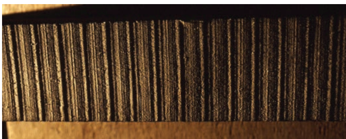
Fig. 7 Traces of a bandsaw on the back of a clock.
