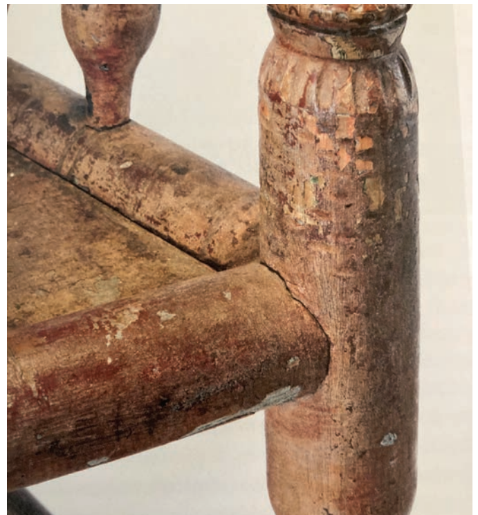
Fig. 10 To carve a concave hollowing of the neck of the tenon cheek to match the surface of a leg of circular cross section demands skill and a sense for accuracy and detailed perfection. Nordiska museet. Photo Peter Segemark.
