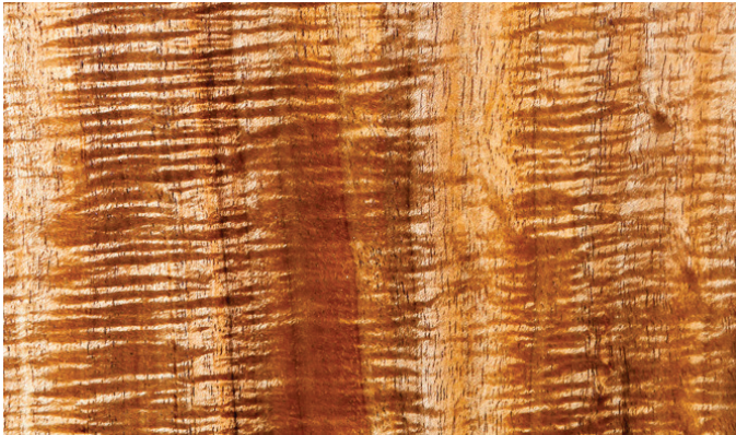
Fig. 2 An example of highly figured Victorian blackwood, sanded to P400 and finished with an oil finish. 2022 © Dunstone Design. Image by Cam Mills.
