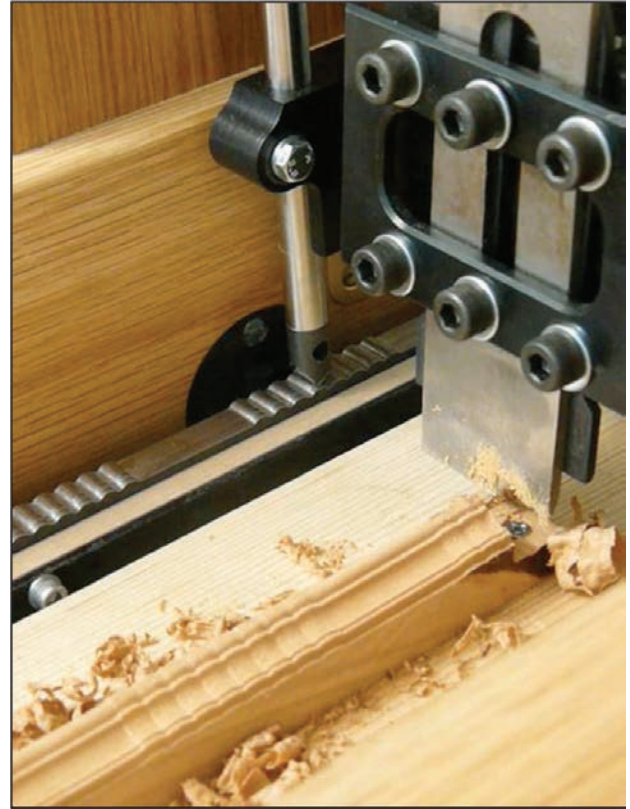
Fig. 2 Manufacturing ripple moulding.
