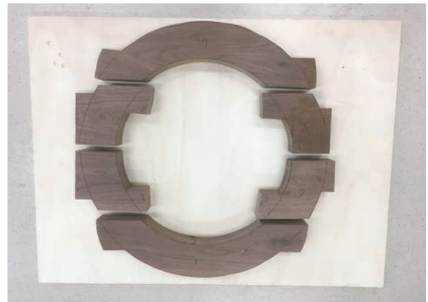
Fig. 5 The separate pieces of the frame with corners for clamping. © The author.
