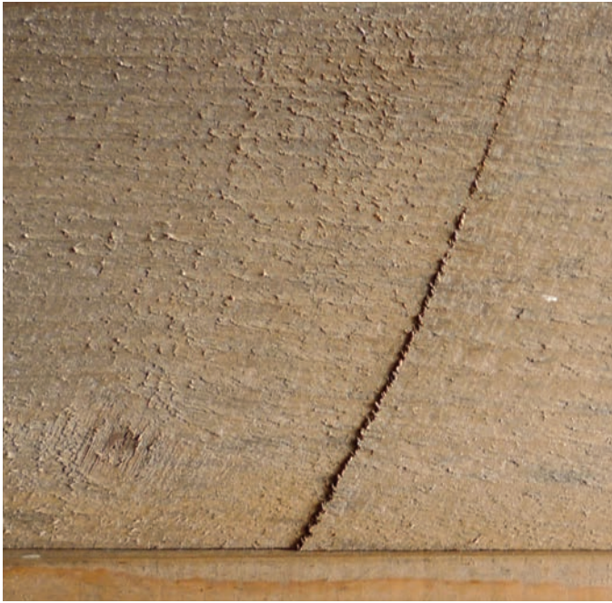
Fig. 8 Traces of a circular saw on the back board of a cupboard. Collection Zuiderzeemuseum, Inv.nr.: 4094 ZZN.
