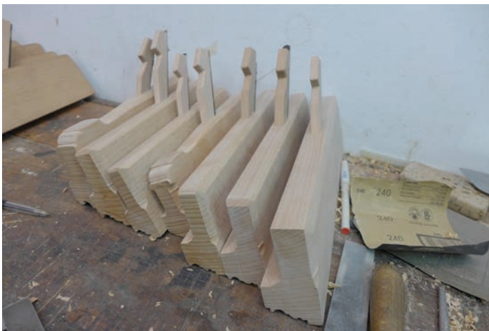
Fig. 7 Replica planes in the process of making. © The authors.
