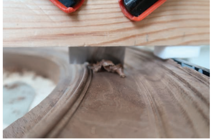
Fig. 11 The scraping in action with the end result, before applying the chalk ground. © The author.
