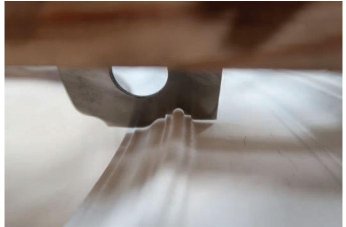
Fig. 13 Scraping the chalk ground layer to recover the crispness in the moulding. © The author.
