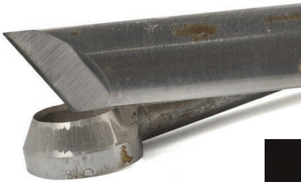
Fig. 6 A sharp tool will focus the force and allow the tool to cut the wood fibers easily and distinctly, leaving a shiny surface.
