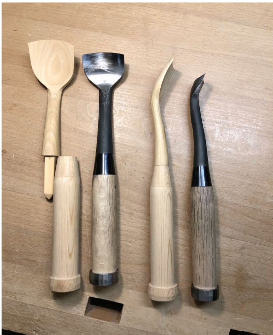
Fig. 7 A model of a special chisel and its finished product. Image by Kenji Komatsu.
