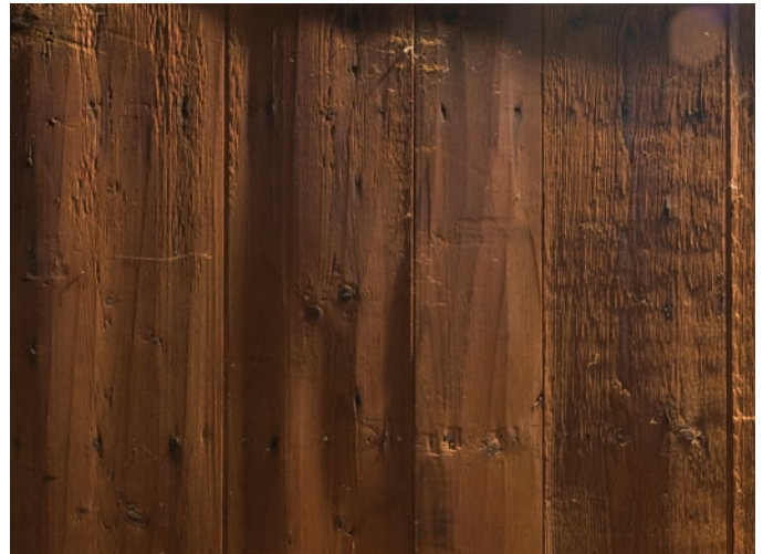
Fig. 6 Traces of a windmill (right) and traces of a scrub plane (left). Back board of a grocery cabinet (1820-1850). Collection Dutch Open Air, Inv.nr.: Museum NOM.32437-61.
