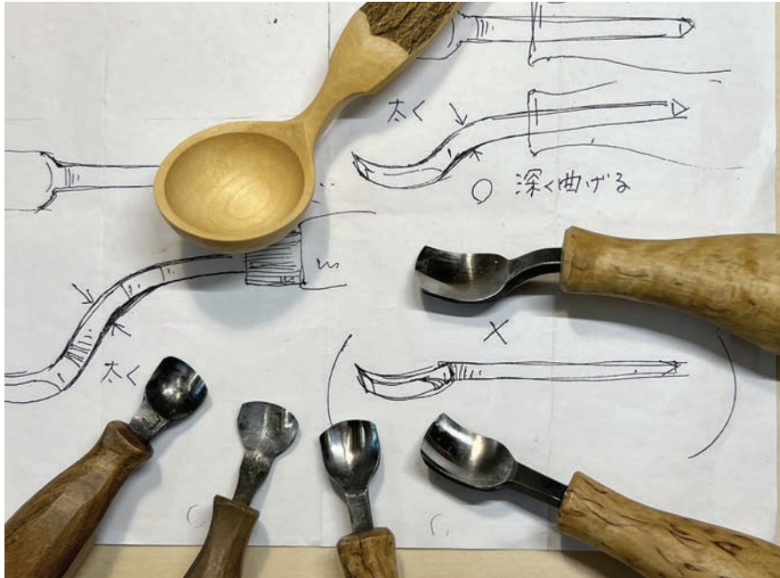
Fig. 6 Tools that have been improved (from left to right) and order drawings, 2018. Image by Kenji Komatsu.
