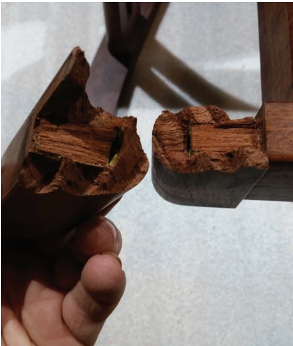
Fig. 5 Broken red gum chair leg on a Seren Chair by Dunstone Design. The short, interlocking grain of the red gum has failed around the tenon.1998. Private collection, Sydney. © Dunstone Design. Image by Evan Dunstone.
