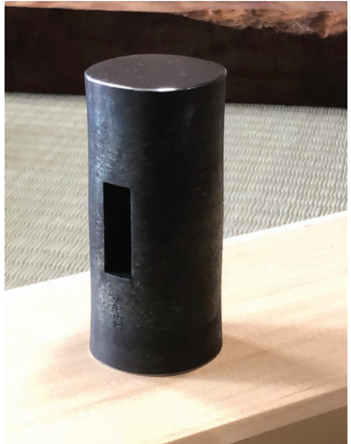
Fig. 9 A 375-gram sledgehammer, Inoue tools shop. Image by Kenji Komatsu.
