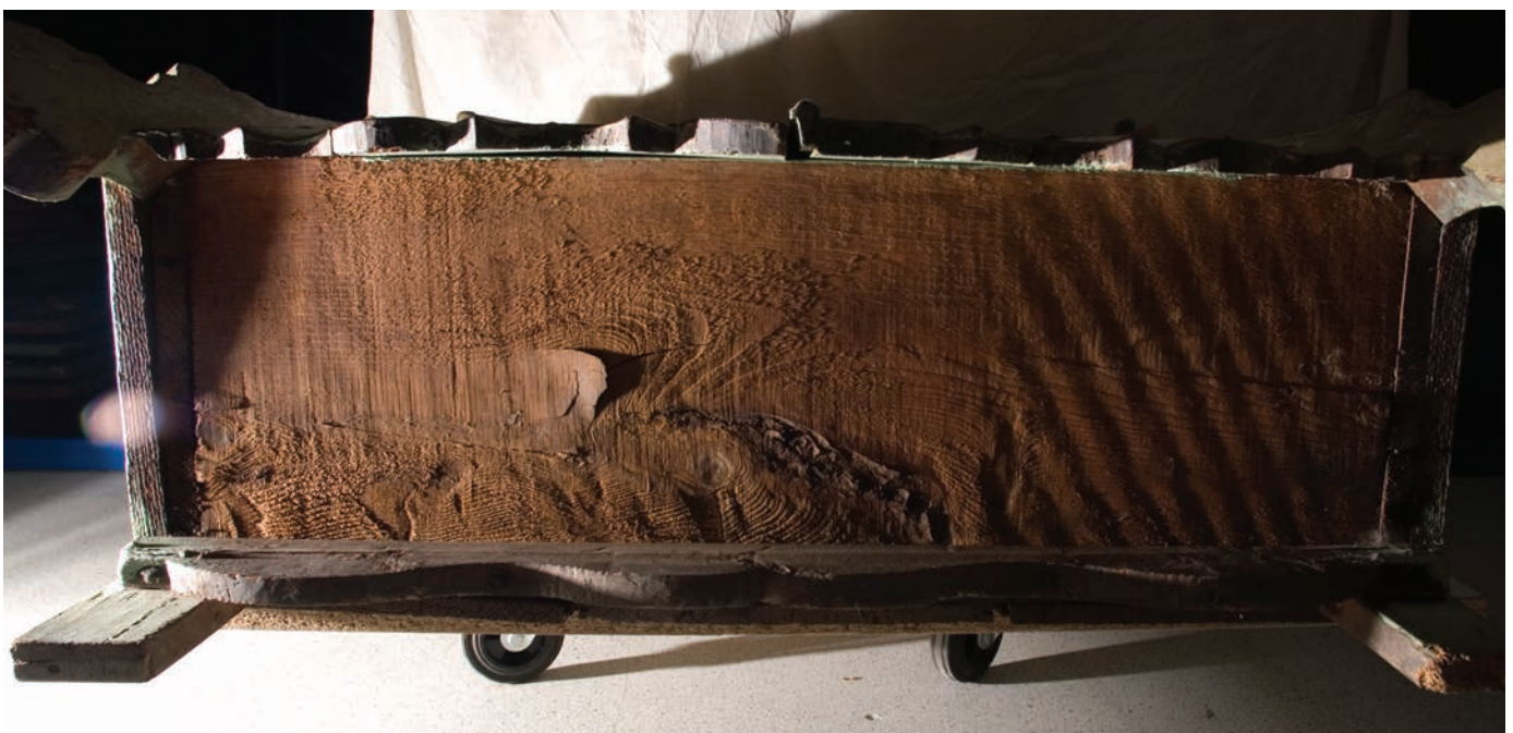
Fig. 5 Traces of a wind saw mill with vibration (right). Bottom of a bureau (1780-1800). Collection Dutch Open Air Museum, Inv.nr.: NOM.5754-46.
