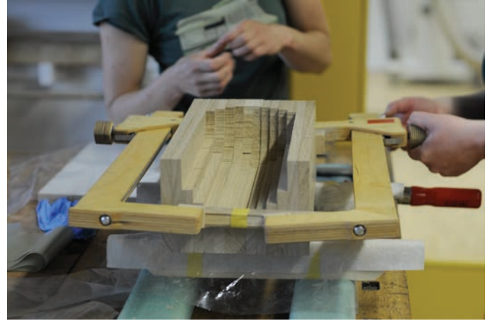
Fig. 7 Gluing up the substructure of the conch. Image by L. Lessinger.
