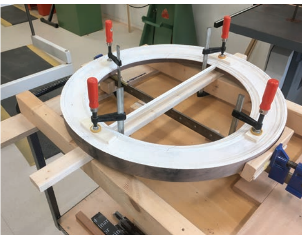
Fig. 18 The backside was gradually pressed into a slight concave position. © The author.
