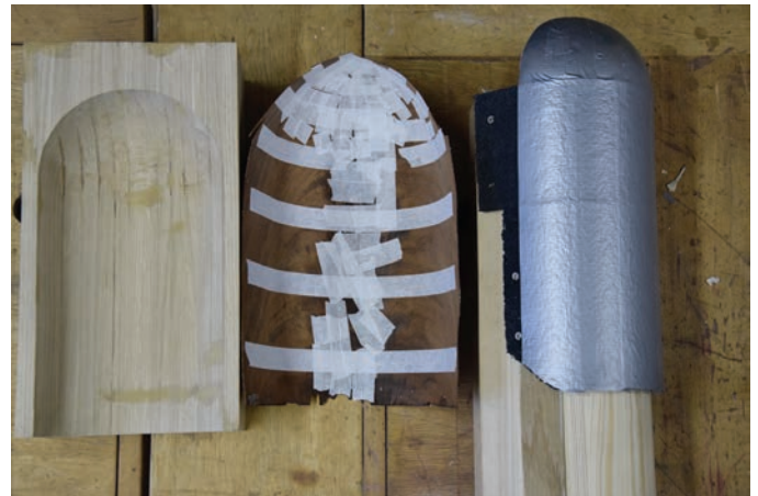
Fig. 9 Veneering using a negative form. Image by L. Lessinger.
