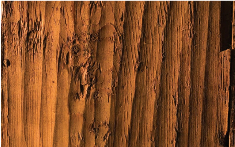
Fig. 10 Scrub plane traces on the back board of a late 17th century cabinet. Collection Zuiderzeemuseum Inv.nr.: ZSM 13183.
