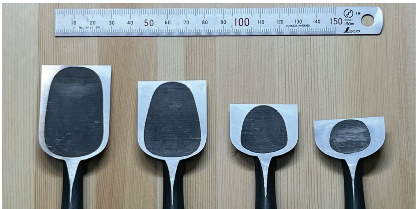
Fig. 4 Appearance of the urasuki remaining on the back even if it was worn out from left to right. Image by Kenji Komatsu.
