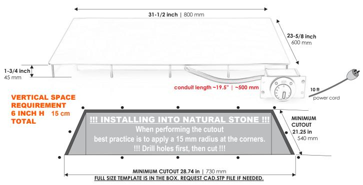
>> The Control Box MUST be firmly fastened to a NON-MOVING surface. Conduit + power cord to be secured.
