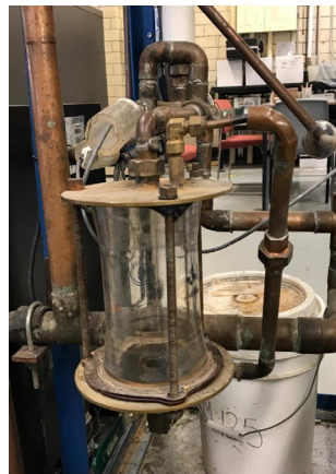
Figure 20. Tube & Shell condensate trap
