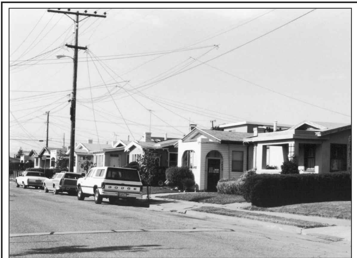
PLATE 24. UNIFORM SETBACKS AND HOUSE SIZES ALONG TENTH STREET IN BERKELEY. Following restrictive covenants written into their deeds, these houses are all 15 feet from the street line. (Credit: Paul Groth)
