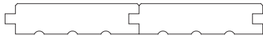
T & G: MICRO-BEVEL Standard on most engineered products, recommended for most prefinished items & wall cladding
