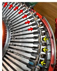
**ADD THE FIRST THREE RIBBER NEEDLES TO THE MACHINE TO LOCK THE DIAL ALIGNMENT:**
