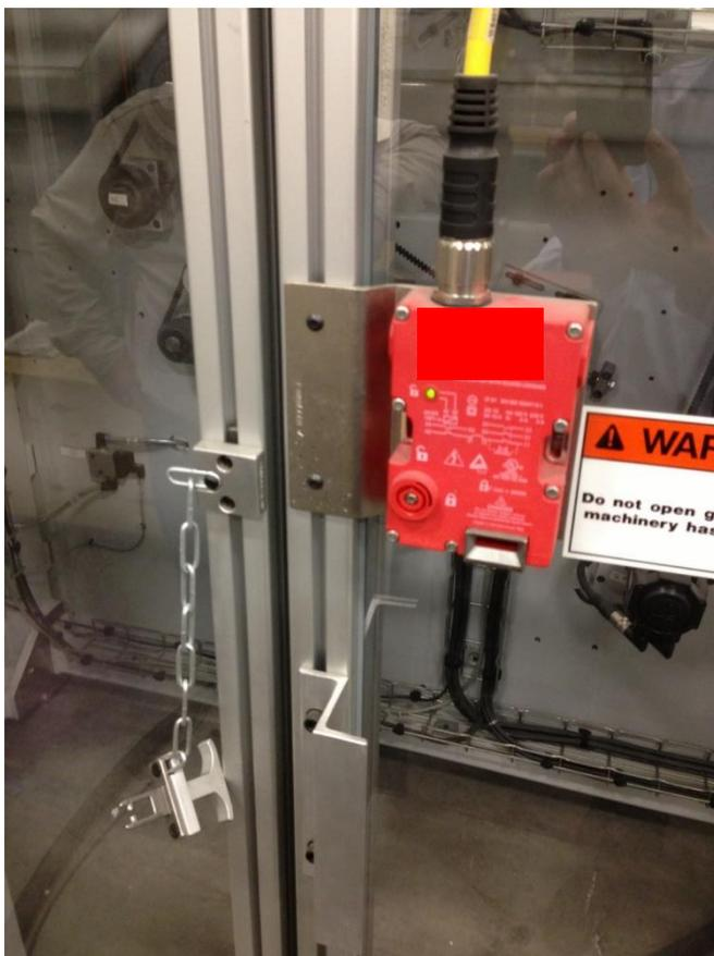
Category 4 rated switch not applied per manufacturer’s requirements or relevant standards, and thus subject to a single point of failure due to mechanical application issues, i.e., chain (breakage) or fastener (single button head screw barely larger than the chain link).
