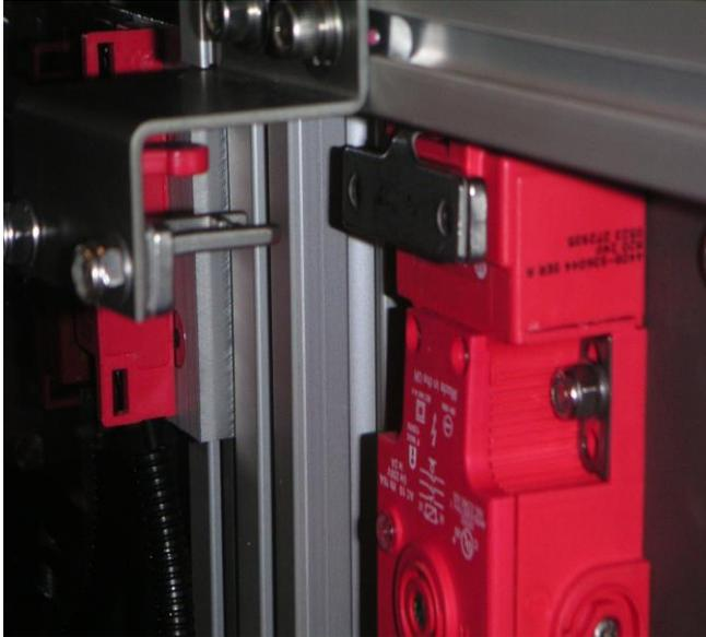
Bypass “cheater key” inserted into switch allows access panel to be opened with the equipment operational and thus defeating the Alternative Method.
