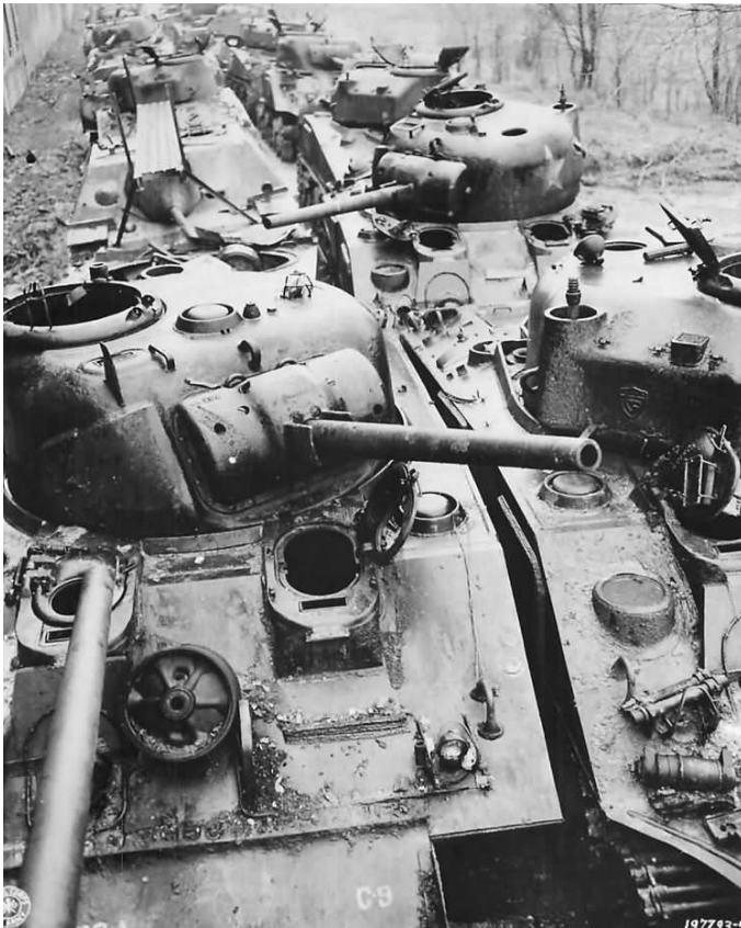
Damaged M4 Sherman tanks await repairs at an ordnance depot in the ETO
