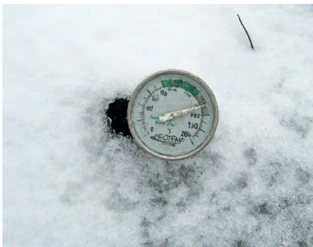
Even during snowy winters, the center of a compost pile can retain temperatures above 100 degrees Fahrenheit.
