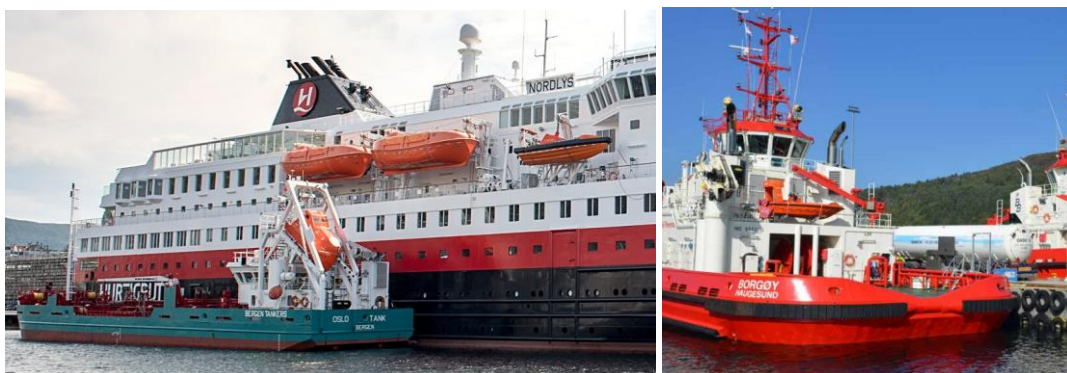
Figure 1-8 Bunkering operations from tanker vessel to Hurtigruten (left – photo: Gasnor/Marit Hommedal) and from road tanker to tug boat (right – photo: Gasnor)
