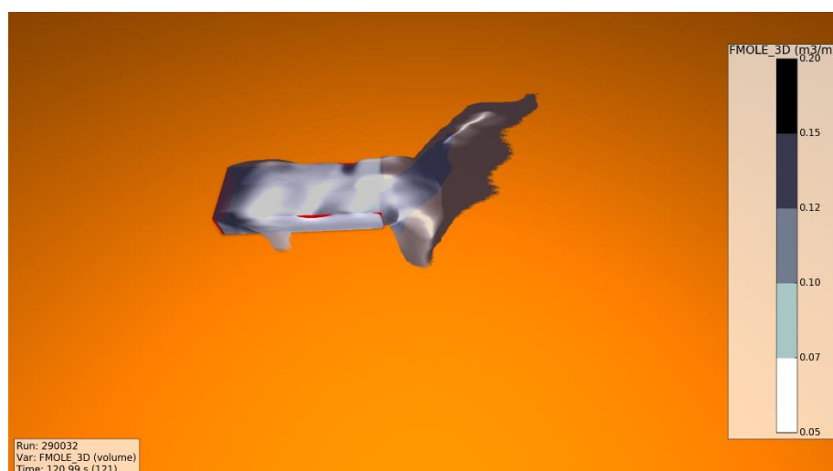
Figure 5-12 Gas dispersion from LNG spray release from 31mm hole (10%) for LNG at minus 150°C, LFL plume shown after 2 minutes.
