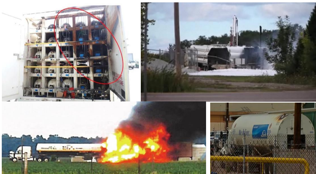
Figure 2-3 Examples of leaks and fires related to transportation of hydrogen, upper plots show compressed gas incidents from in Los Angeles, California, 2018 (left) and Rochester; New York, 2010 (right) while lower plots show incidents with fires in LH2 trailers in Ohio, 2015 (left) and El Cajon, California, 2018 (right).
