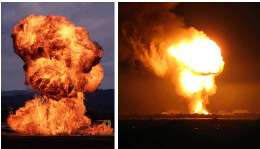
Figure 2-9 BLEVEs in hydrogen and ammonia would likely have quite different characteristics from each other, and from propane BLEVEs. Left photo shows propane BLEVE testing at Queens University, Canada, right photo shows Sunrise BLEVE-accident in Toronto (2008).
