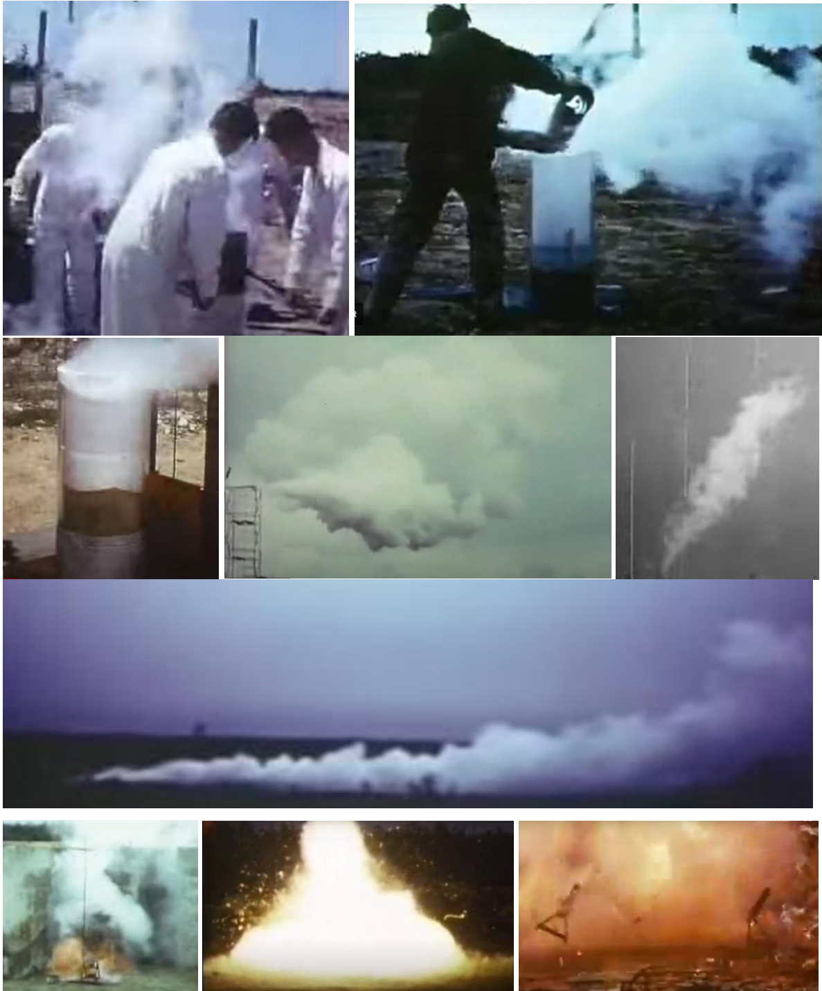
Figure 2-10 Very impressive test program into LH2 hazards by AD Little Company for US Air Force in 1960 studying release, dispersion, deflagration and detonation. The test procedures may give the impression that LH2-handling is free of hazards, which is far from the case.
