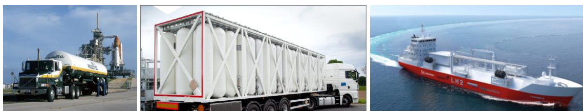
Figure 1-6 Transportation of hydrogen and ammonia in Norway can be expected done primarily by liquid road tankers or compressed gas trucks or by ship, photos: Air Products (left), Hexagon (middle) and Wilhelmsen (right).
