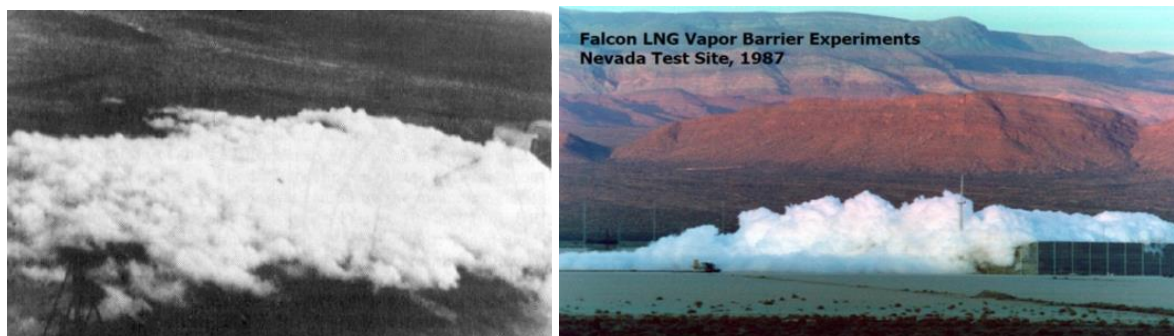
Figure 2-15 LNG release tests from Burro experiments (left) and Falcon experiments (right).
