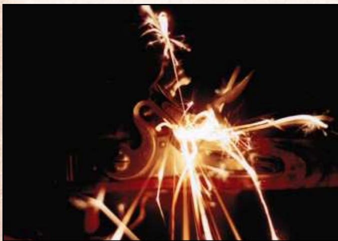
Fig. 8. A lock that throws a shower of sparks like this has no perceptible lag time between hammer fall and ignition.
