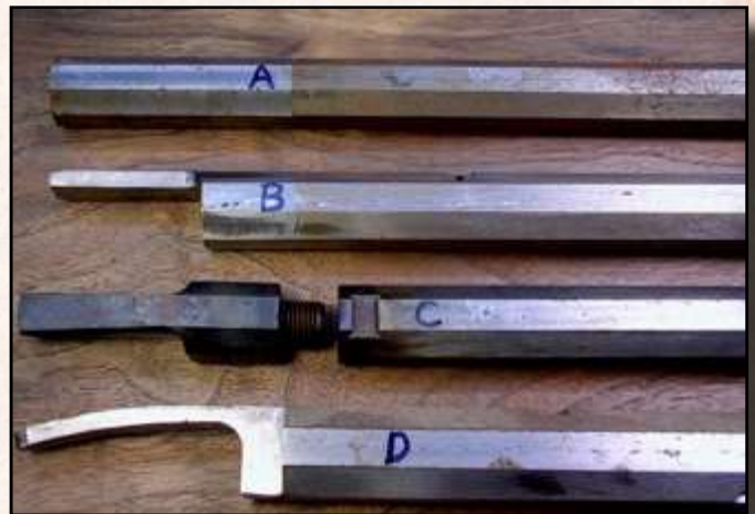
Fig. 4. A custom breech begins with round stock threaded to mate tightly against the inside shoulder of the barrel and also against its exterior. The blank is then milled to match the barrel (a). The excess metal is then removed from the tang area. (b). The tang is heated red-hot and hammer forged to its rough dimensions. (c). Note that the custom breech does not have a lug. (d) that will interfere with the placing of the rear lock bolt.
