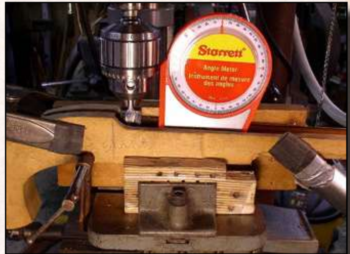
Fig. 6. An inclinometer can be purchased from any building supply store. It can measure deviation from level down to 1/2°.
