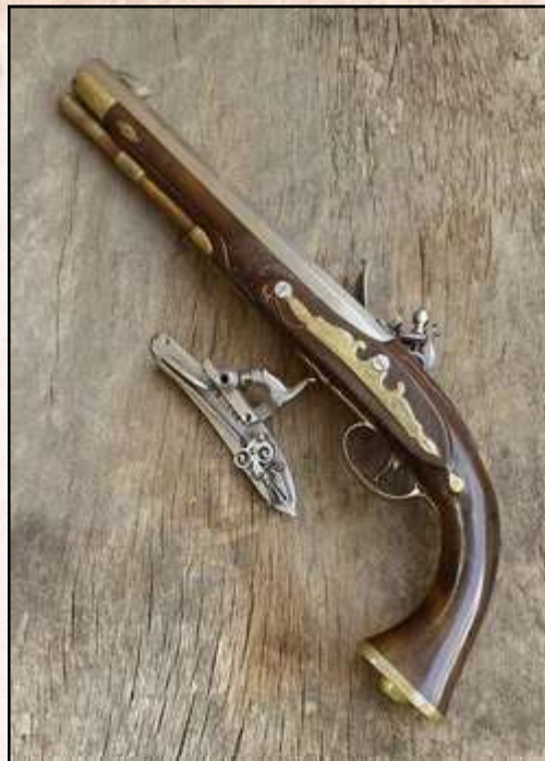
Fig. 13. The butt of this pistol terminates in a pronounced flare that resists muzzle droop as it comes up against the heel of the hand
