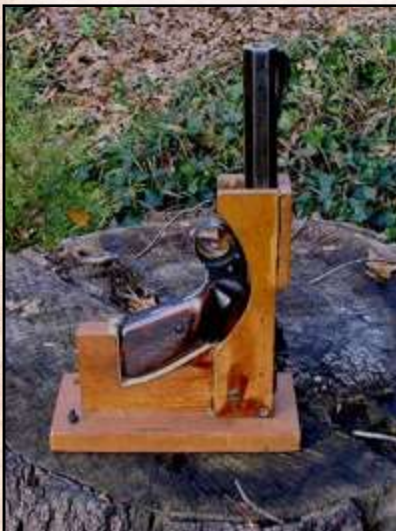
Fig. 2. This pistol stand made from scrap wood was very handy for loading at the range.
