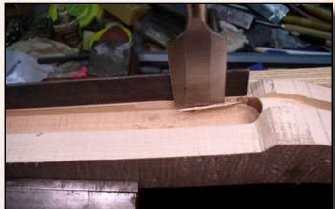
Fig. 7. Inletting a tapered or swamped barrel can be tedious, but what is worse is leaving a wood-to-metal gap. Go slowly, working back and forth on both sides of the channel.
