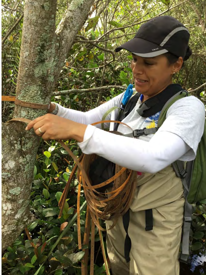
LILA scientists installing tree bands to measure the growth rate (diameter) of trees as the experimental LILA tree islands experience flooding. Photo credit: Kelsey Pollack.
