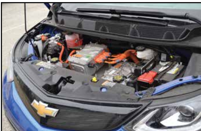
The Chevy Volt features a high voltage system, which contains nine individual components working together.
