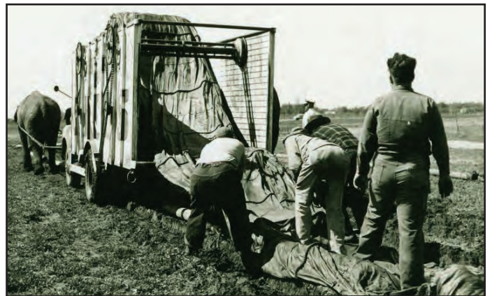
Many local businesses also partnered with the show owners to innovate and mechanize the processes required to move the circus from town to town. Shown above is the motorized canvas spool that was mounted to a semi-tractor, and allowed the big circus tent to be folded and spooled into a large truck making it possible to load and unload the large tents every day.
