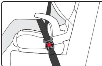
5. Remove slack from the vehicle belt.
