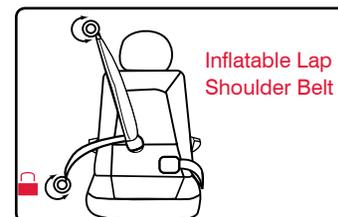
**NOTE:** To use a child seat with this type of vehicle belt, you will need to switch the retractor for the lap section of the seat belt to the ALR mode.
