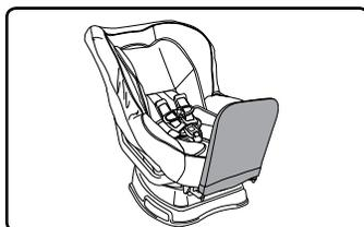
3. Recline the unoccupied child seat to position 3 and place rear-facing on the vehicle seat (see page 24). Ensure that no more than 7.6 cm (3 in.) of the base hangs over the edge of the vehicle seat.
