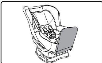
3. Recline the unoccupied child seat to position 3 and place rear-facing on the vehicle seat (see page 24). Ensure that no more than 7.6 cm (3 in.) of the base hangs over the edge of the vehicle seat.
