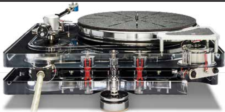
ABOVE: Transparent rear of the SG-1 reveals 7-pin DIN connector for the Imperium PSU's dedicated motor link cable [right] and captive tonearm cable with strain relief [left]. Note adjustable 'wings' on the tonearm counterweight for fine azimuth tuning
