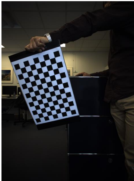
Figure 4: One of the images of a checkerboard used to calibrate camera.
