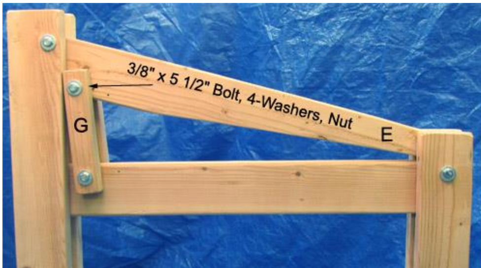
13. Raise part G and connect to handle E using a 3/8" (10 mm) x 5 1/2" bolt, 4-washers and a nut.
