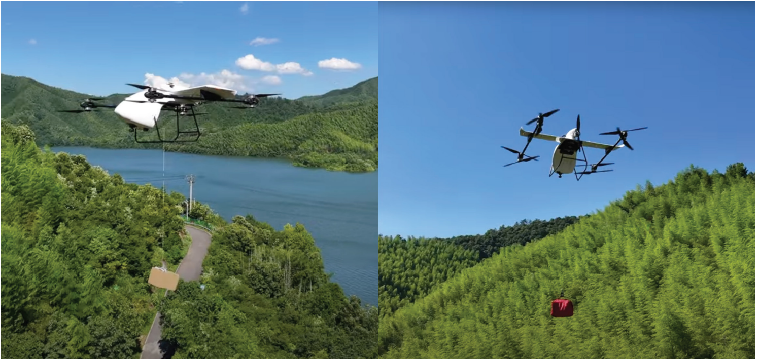
A purpose-built commercial drone winch enables payloads to be deposited from altitude where spinning propellers are kept far from people, property, and potential ground obstructions.
