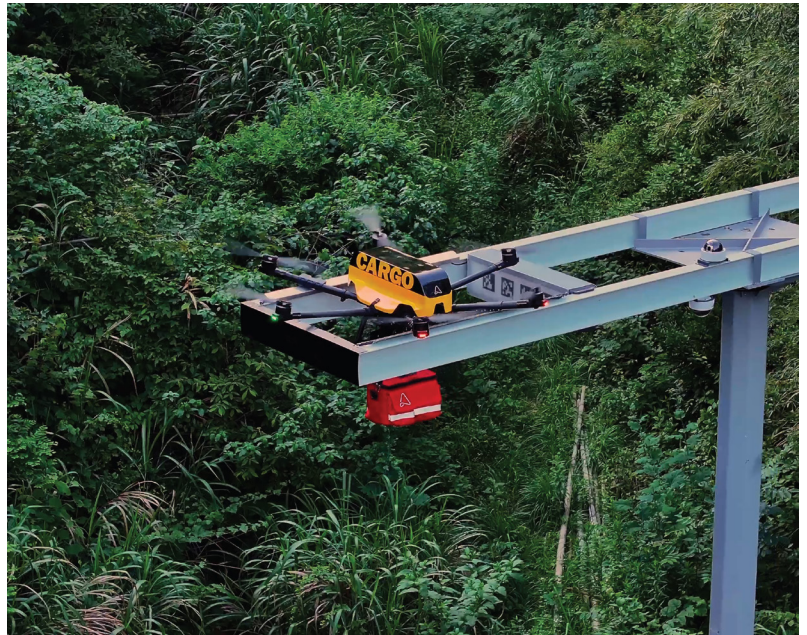
A purpose-built commercial drone winch enables payloads to be deposited from altitude where spinning propellers are kept far from people, property, and potential ground obstructions.
