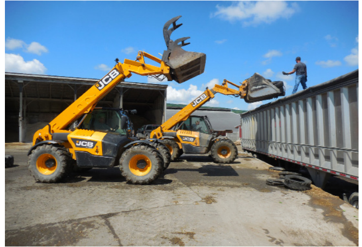
Telescopic handlers loading tires into semi-trailer
