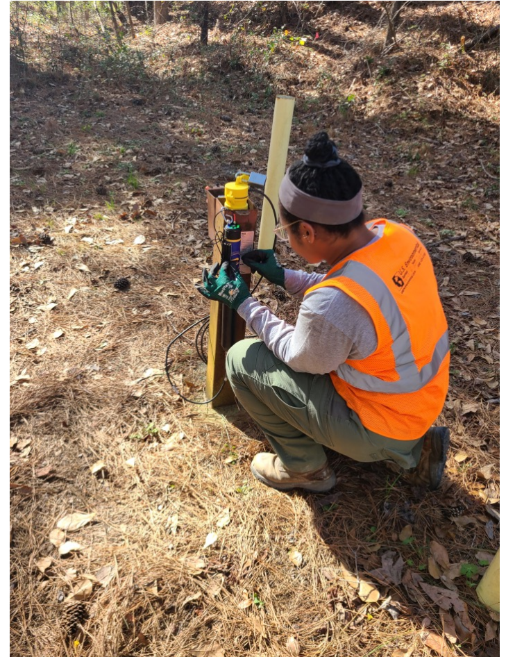
Monitoring well measurements during semiannual groundwater sampling
