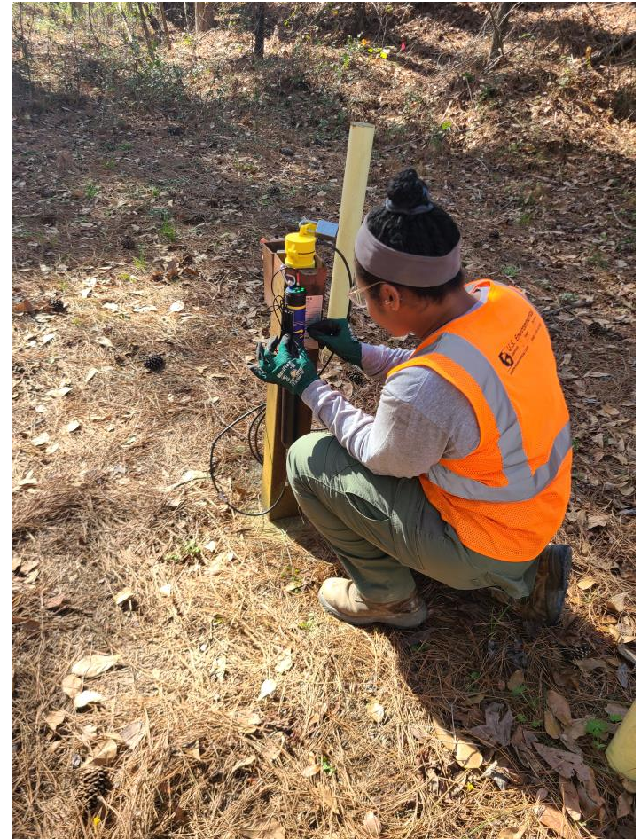
Monitoring well measurements during semiannual groundwater sampling
